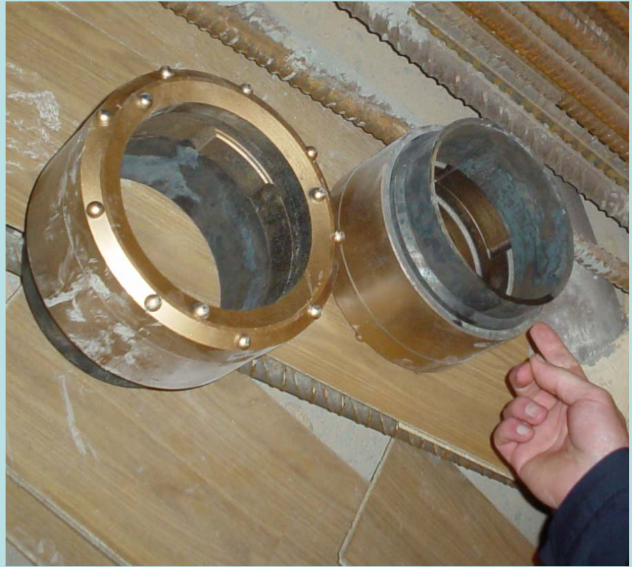
Ring crown – welded to tube, left at tip
