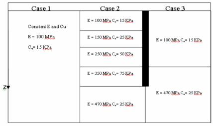
Soil density  $\rho{=}1760~kg/m^3$  and Poisson's Ratio  $\nu{=}0.48$  for all soil layers.
