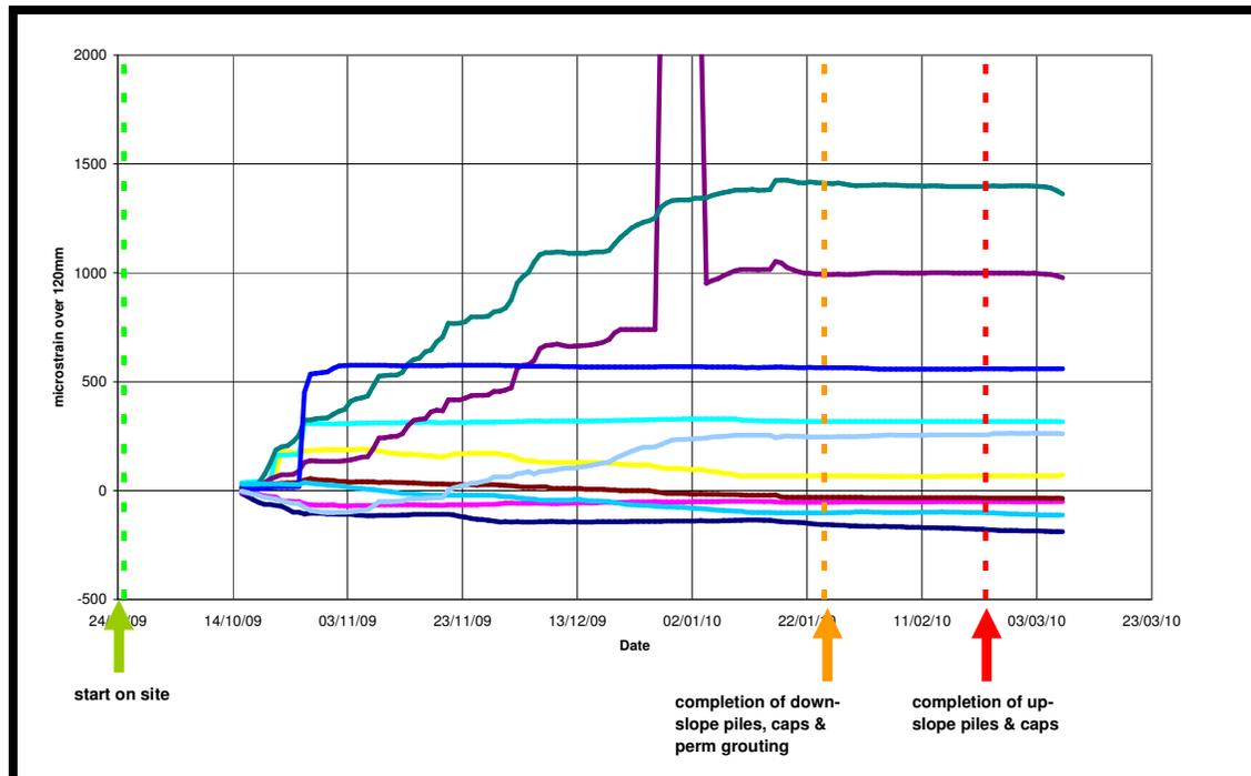
Figure 13: Strain gauge results, measured inside the conduit, across existing cracks.
