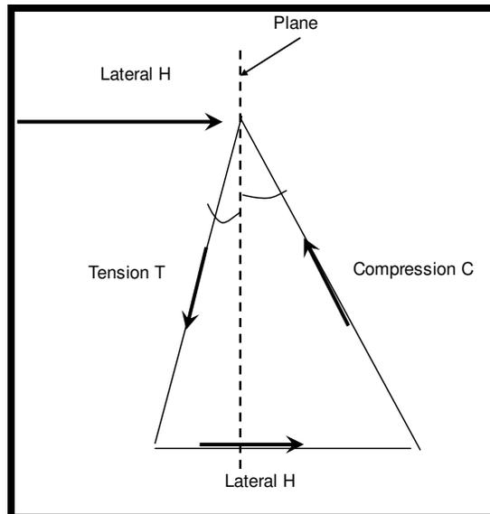
Figure 10. Triangle of forces used to estimate micropile axial loads
