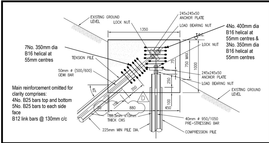
Figure 11. Pile cap detail
