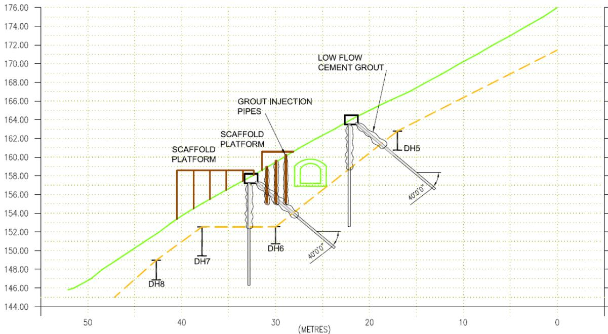
Figure 7. Typical section through slope stabilisation works
