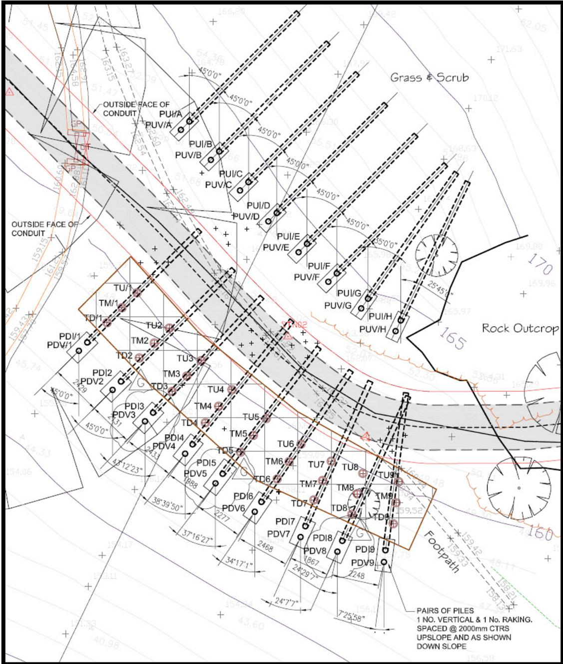
Figure 12. Stabilisation works layout
