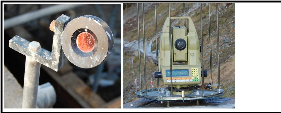
Figure 5. Automated monitoring system – prism and total station
