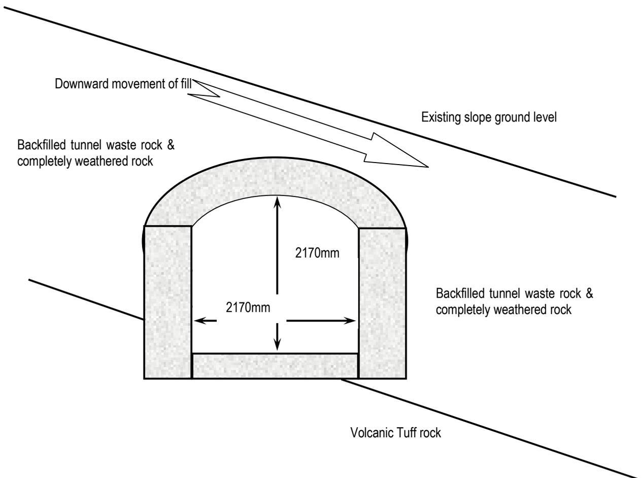
Figure 3. Typical cross section through mass concrete conduit at Nab Scar
