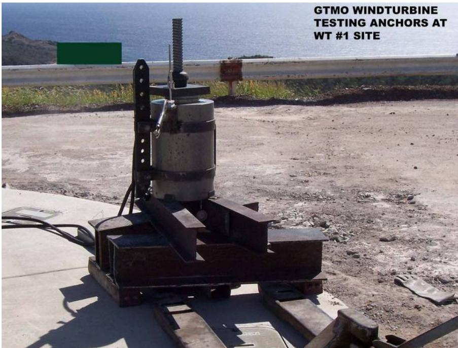
Figure 27, Testing and Post-Tensioning of Hollow Core Micro Piles
