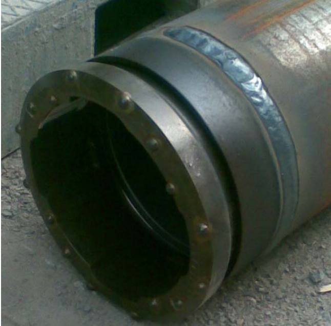
Figure 2. Ringset at the point of a RD-pile, RD-270.
