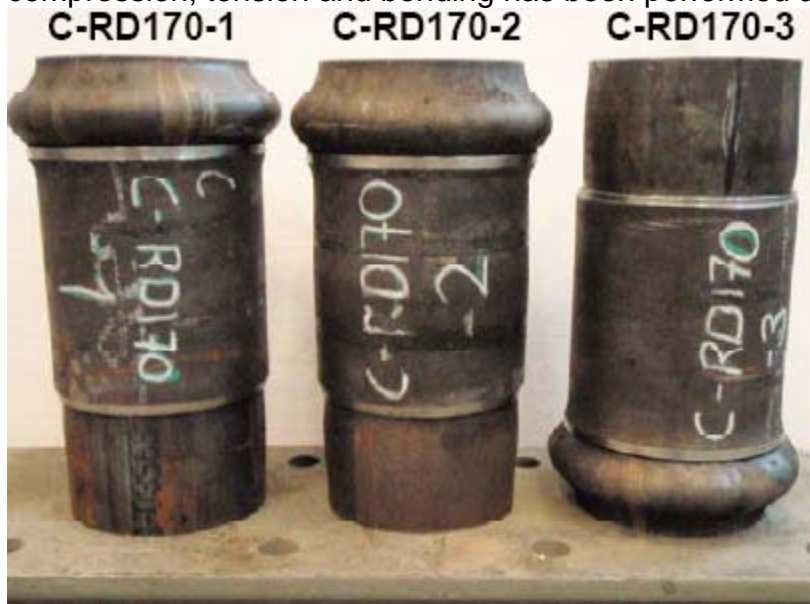
Fig 4. RD-pile splices tested to ultimate compressive capacity, RD170/10.
