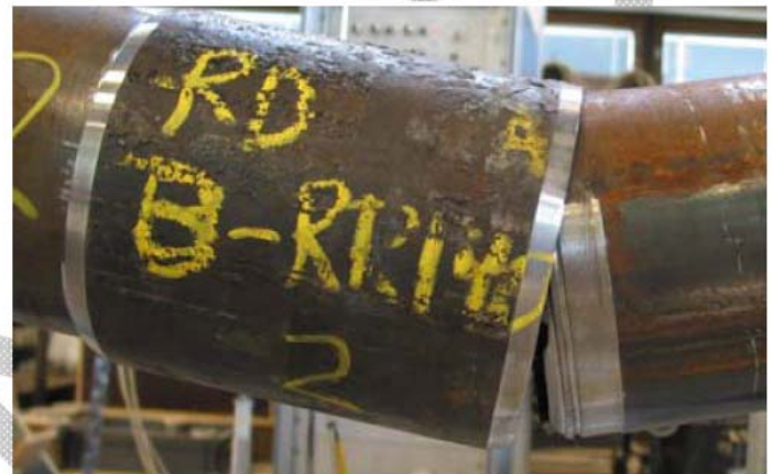
Figure 5.16 Failure of B-RD140-2.
