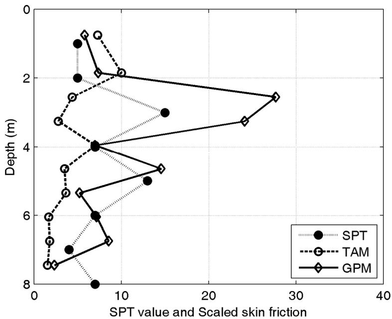
Figure 8. SPT value and scaled skin friction at ultimate loading stage.
