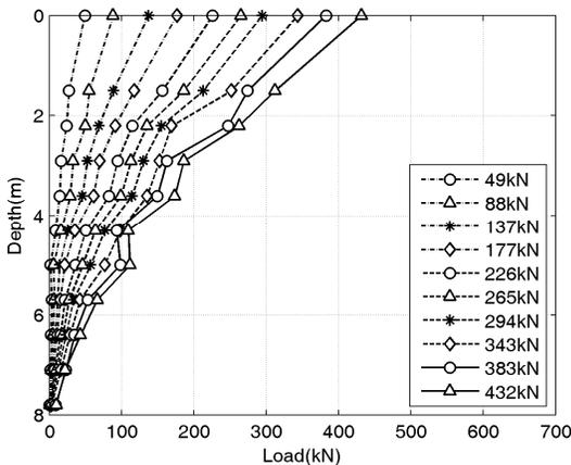
Figure 4. Load transfer behavior for TAM
