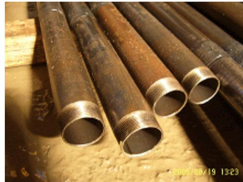
(b) Hollow steel pipe for GPM
