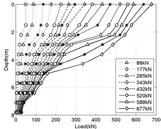
Figure 5. Load transfer behavior for GPM
