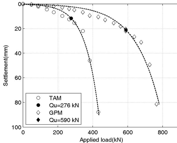
Figure 6. Load vs. displacement curves for the two types of micropiles.
