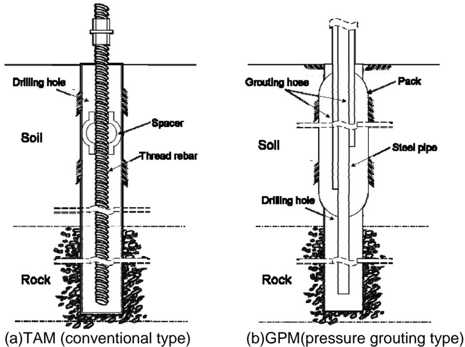
Figure 1. Schematics of two type of micropiles
