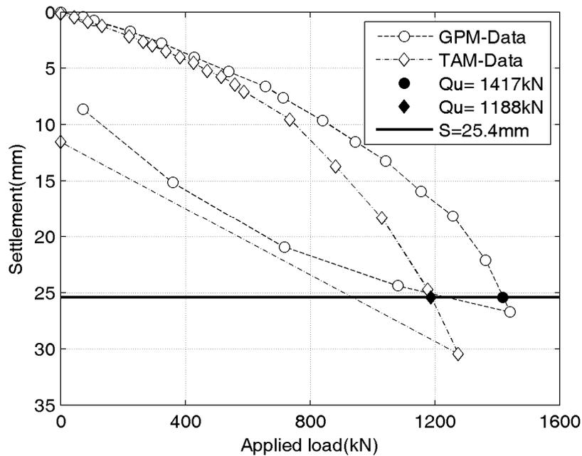
Figure 9. Load vs. Settlement results for Test Set 2
