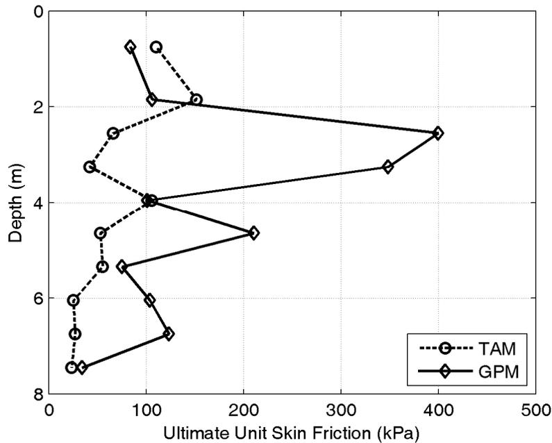
Figure 7. Unit skin friction along depth when ultimate compressive loading was applied
