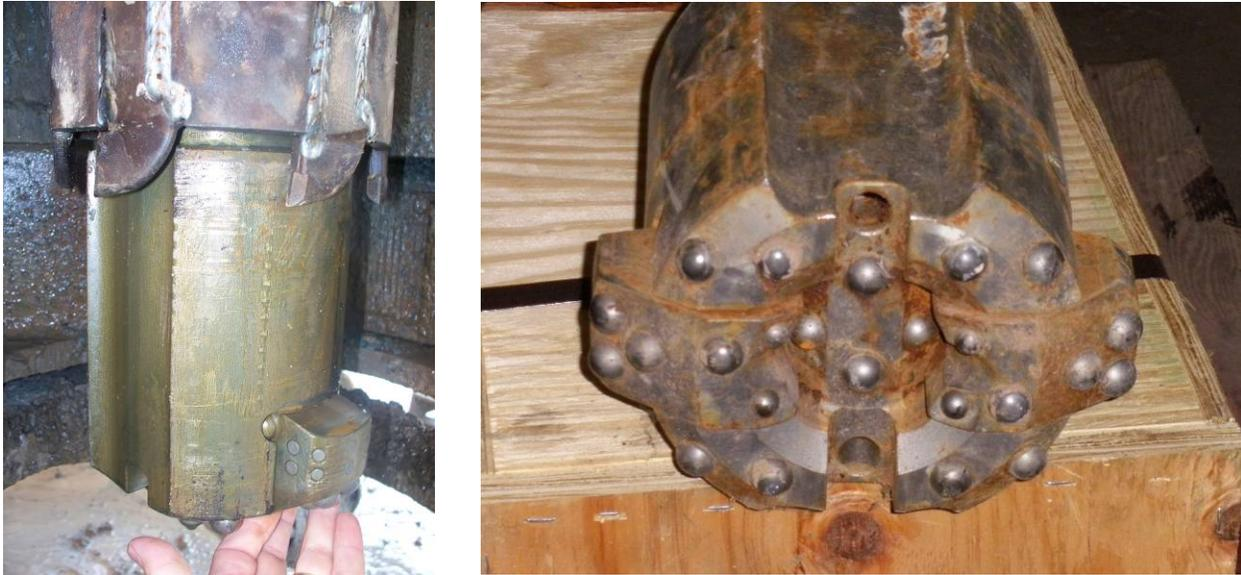
**Figure 4. NUMA Superjaws concentric overburden drilling system**
