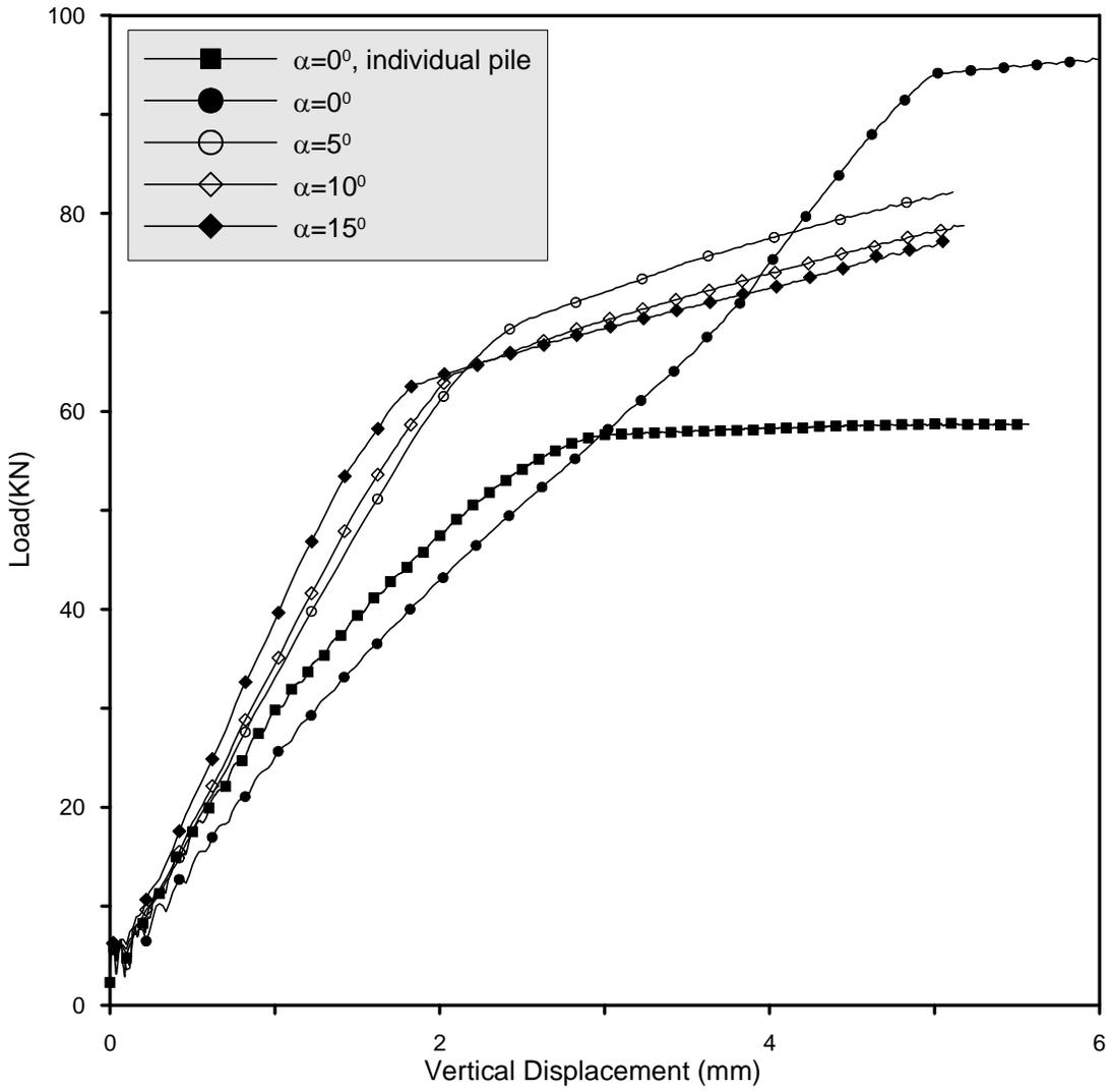
Figure 3a Side Resistance Variation with Network Pile Outward Inclination ( $\psi=-0.1$ )
