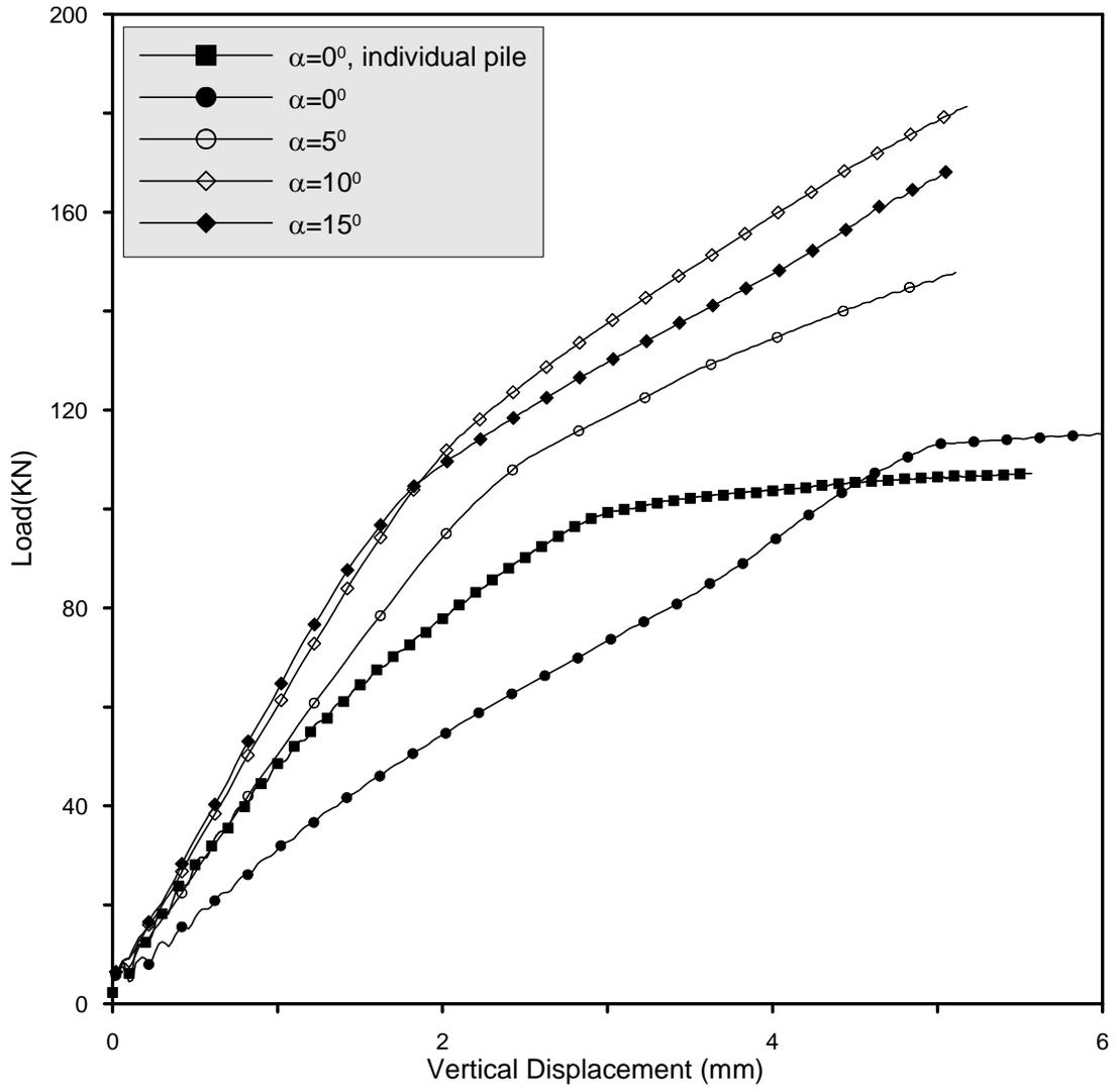
Figure 3c Total Resistance Variation with Network Pile Outward Inclination ( $\psi=-0.1$ )
