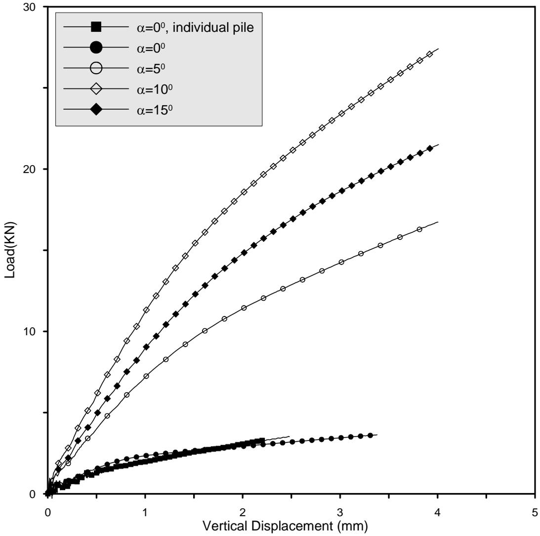
Figure 5b Tip Resistance Variation with Network Pile Outward Inclination ( $\psi=0.1$ )
