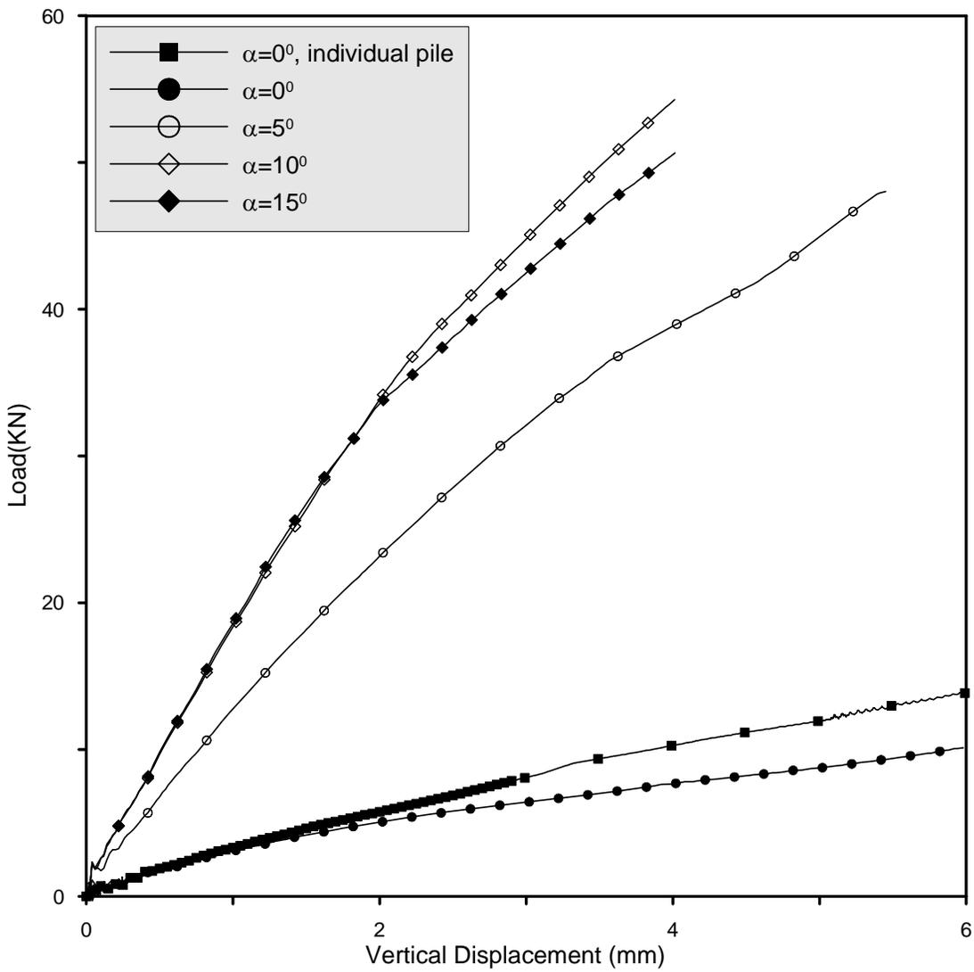
Figure 4b Tip Resistance Variation with Network Pile Outward Inclination ( $\psi=0.0$ )
