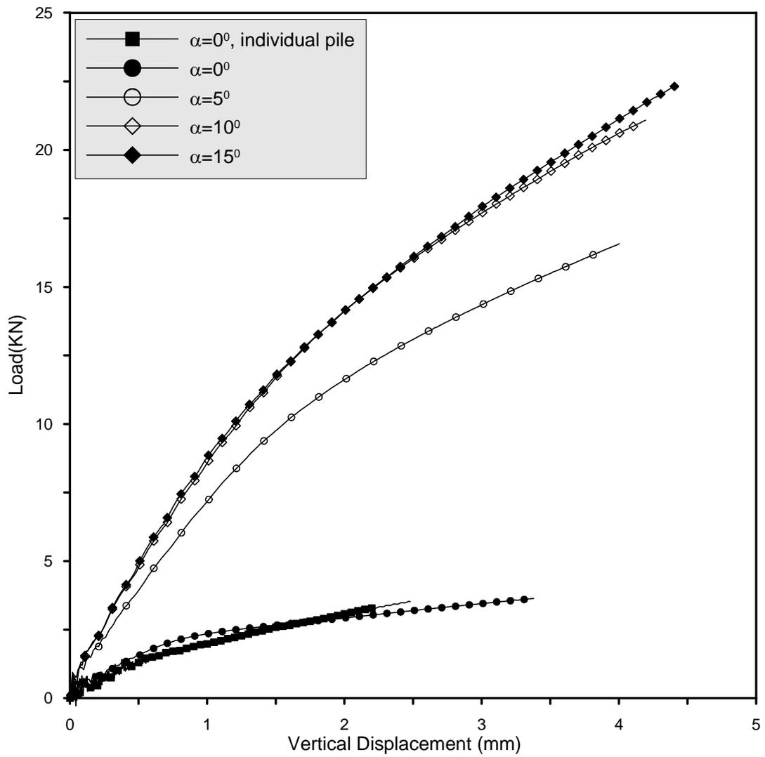
Figure 8b Tip Resistance Variation with Network Pile Inward Inclination ( $\psi=0.1$ )
