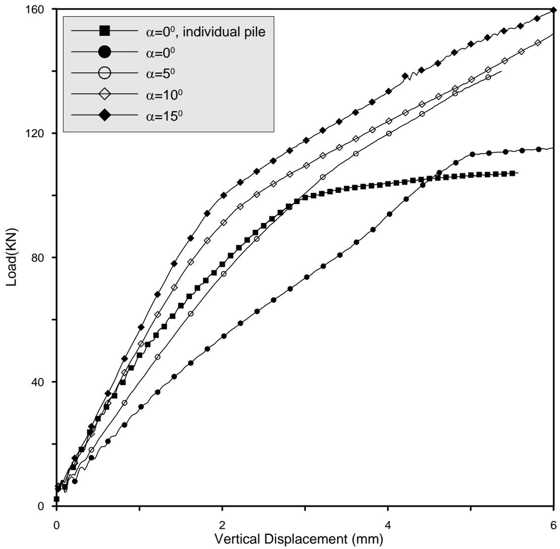
Figure 6c Total Resistance Variation with Network Pile Inward Inclination ( $\psi=-0.1$ )
