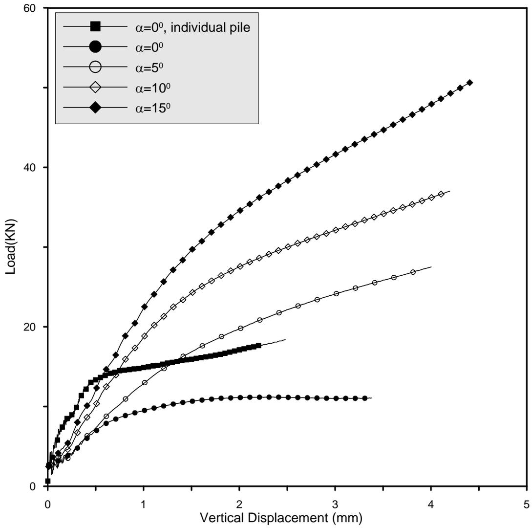
Figure 8a Side Resistance Variation with Network Pile Inward Inclination ( $\psi=0.1$ )
