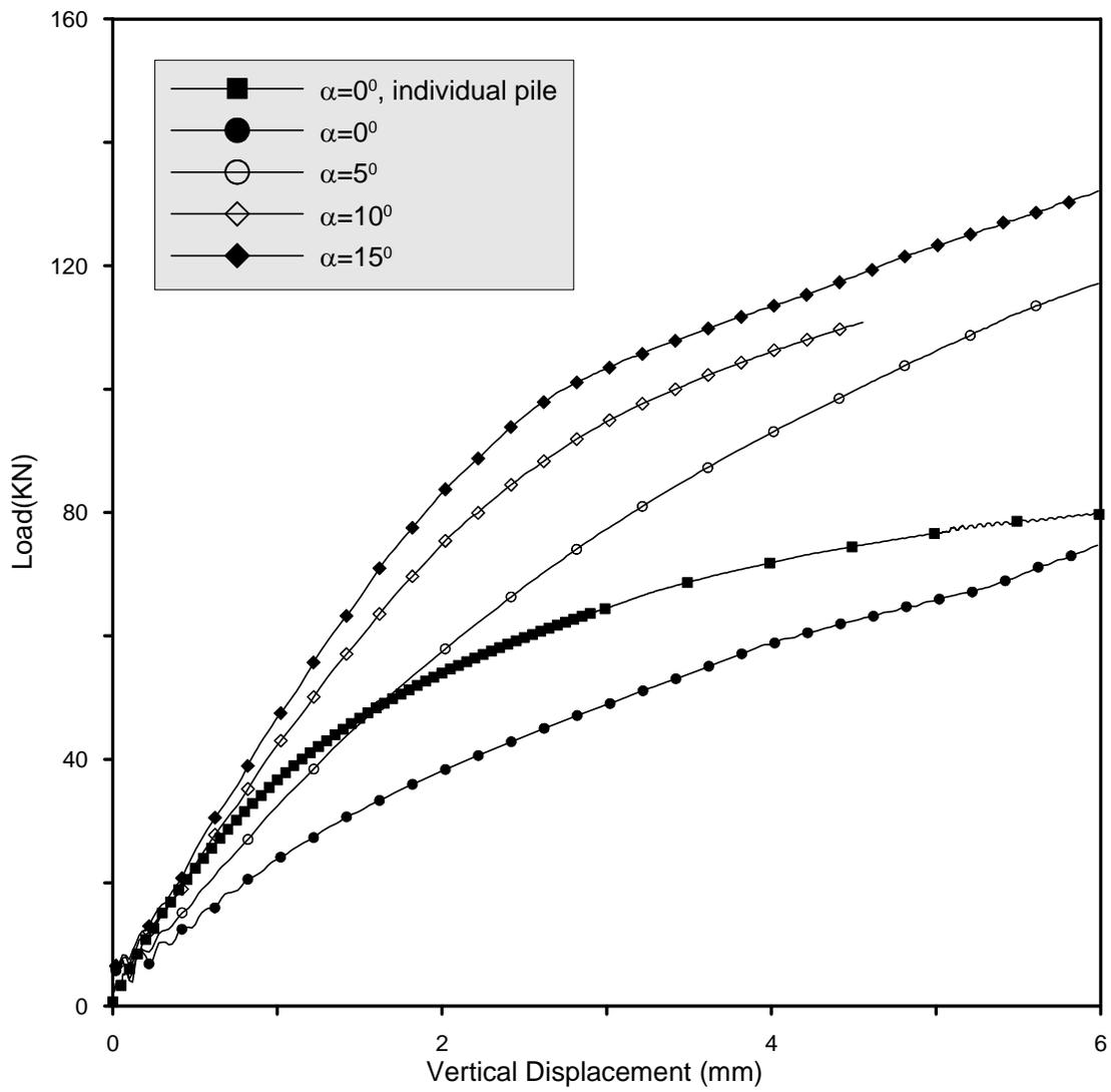
Figure 7c Total Resistance Variation with Network Pile Inward Inclination ( $\psi=0.0$ )
