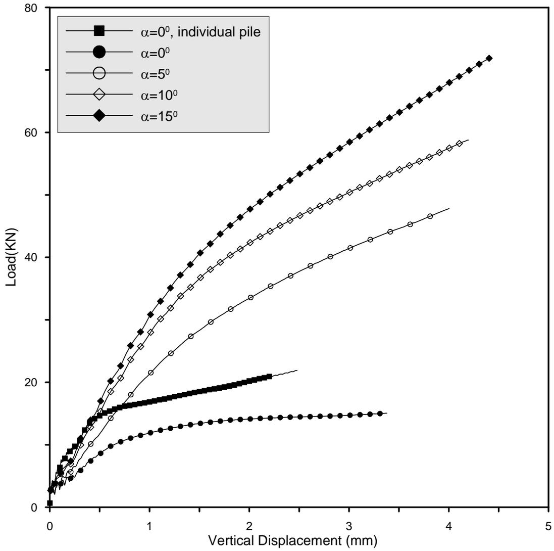
Figure 8c Total Resistance Variation with Network Pile Inward Inclination ( $\psi=0.1$ )
