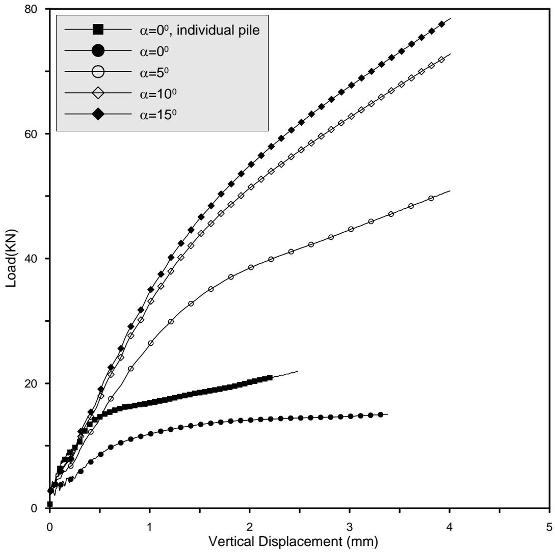
Figure 5c Total Resistance Variation with Network Pile Outward Inclination ( $\psi=0.1$ )
