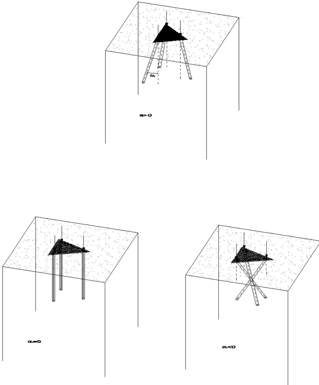
Figure 2: Model setup for network Micropiles
