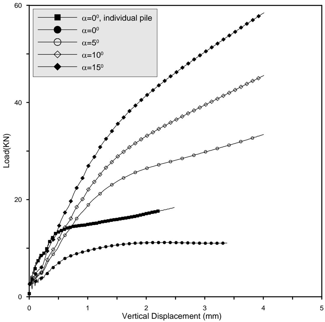
Figure 5a Side Resistance Variation with Network Pile Outward Inclination ( $\psi=0.1$ )
