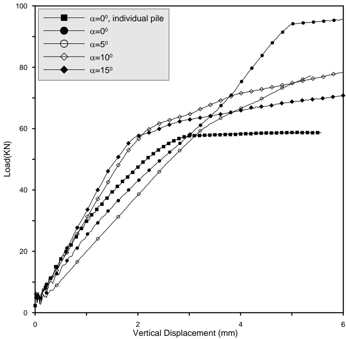
Figure 6a Side Resistance Variation with Network Pile Inward Inclination ( $\psi=-0.1$ )
