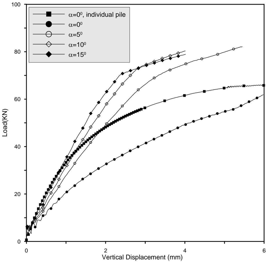
Figure 4a Side Resistance Variation with Network Pile Outward Inclination ( $\psi=0.0$ )
