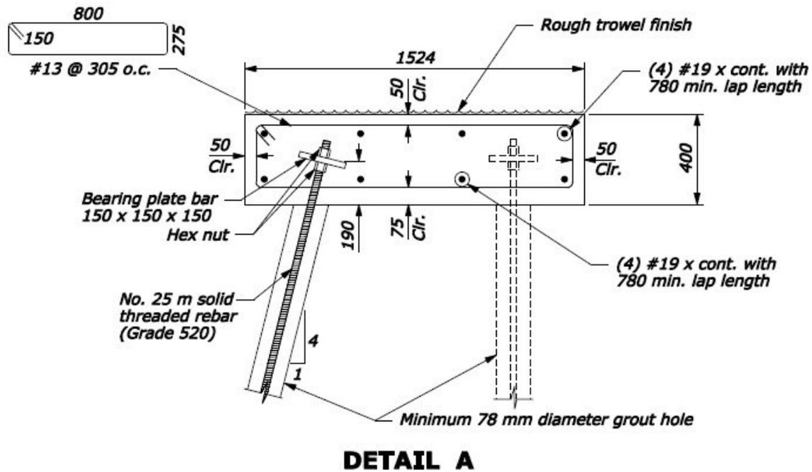
Figure 5 – Micropile Cap Typical Detail
