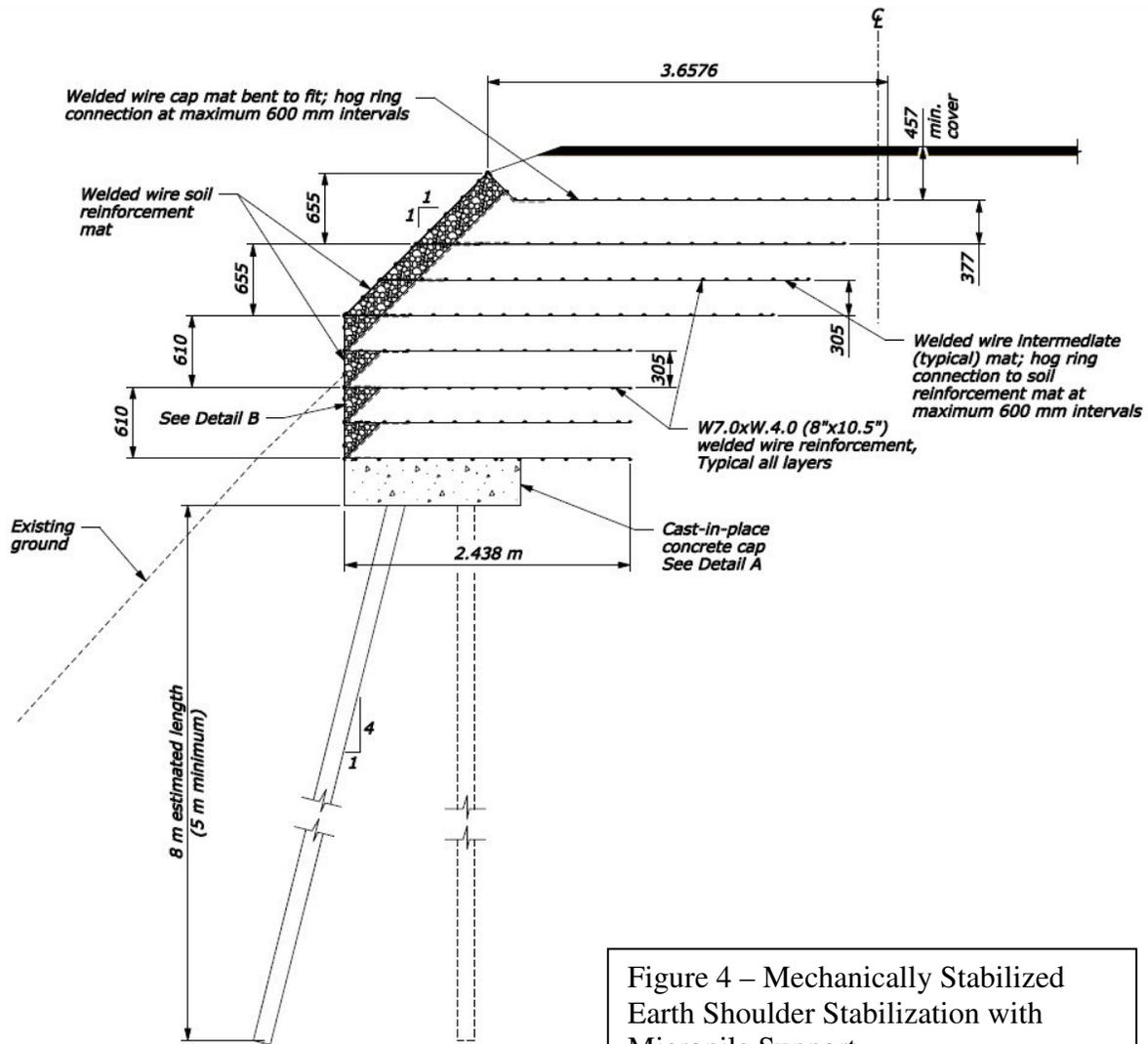
Figure 4 – Mechanically Stabilized Earth Shoulder Stabilization with Micropile Support
