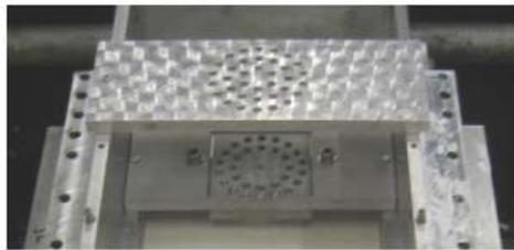
Guide plate, pile cap holder and pile cap
