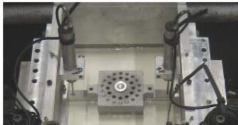
Pile cap, LVDT brackets and LVDTs
