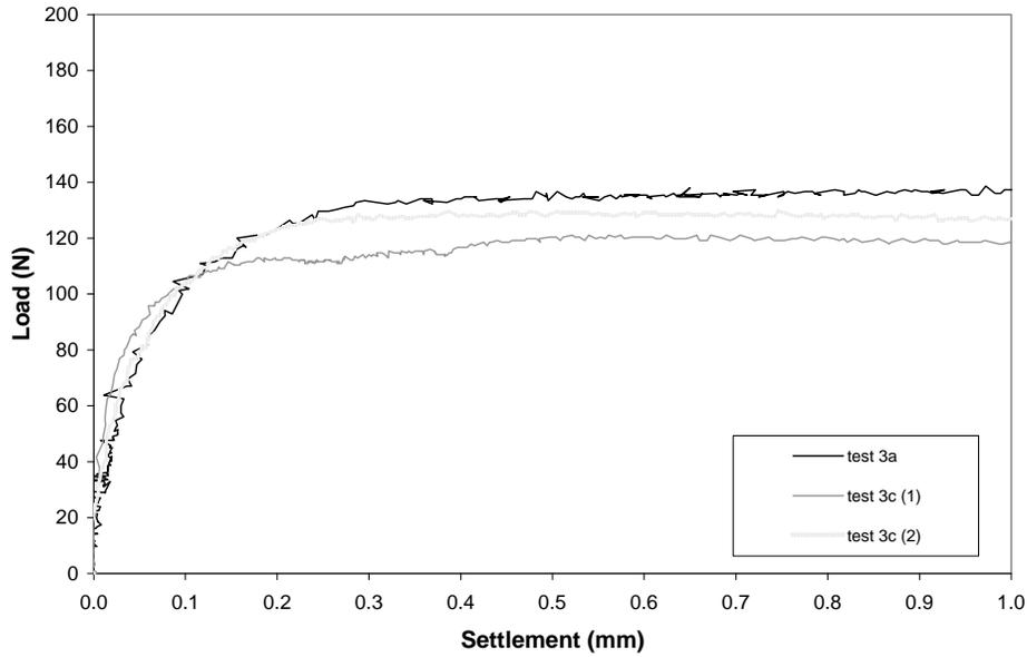
Figure 7. Results from single pile tests
