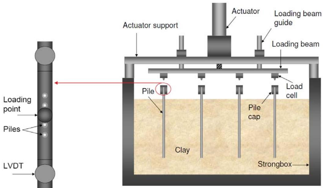
Figure 4. Long section of strongbox and plan view of pile cap
