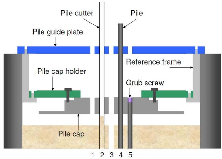
1. Apparatus in place pre pile installation
