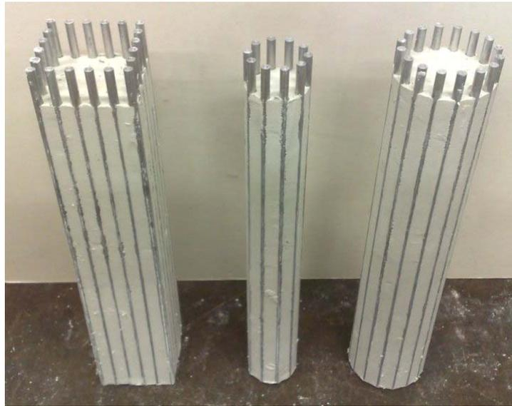
Figure 1. Circular and square perimeter groups after excavation from the clay sample
