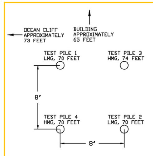
**Figure 11: Test Pile Layout**
