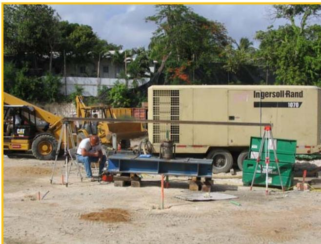
**Figure 10: Micropile Tension Testing**
