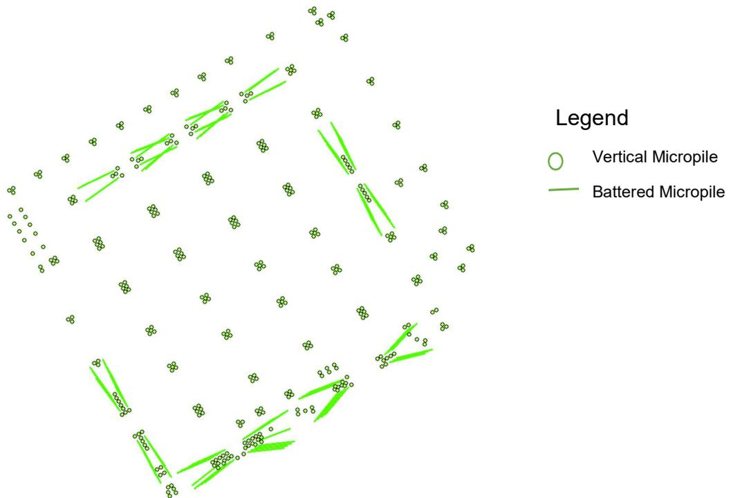
Figure 2. Revised pile layout with 1 to 2 piles removed per pile cap.
